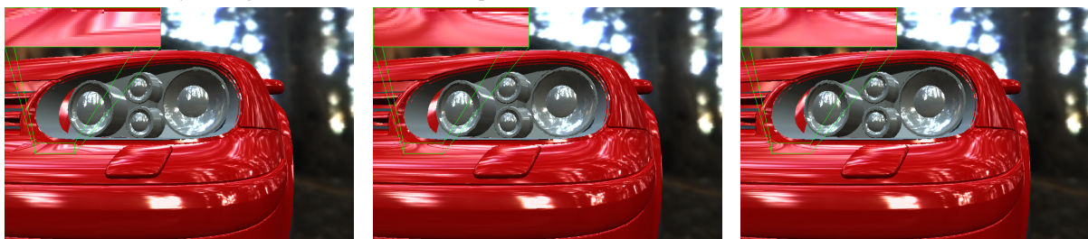
Figure 10: A frame from the golf video sequence showing the results of standard tessellation (left), normal maps (middle) and appearance preserving tessellation (right). Note that although the reflections seem to be correct for the normal map method, they are all shifted due to the discretization of the normals leading to false conclusions or even fake discontinuities.
