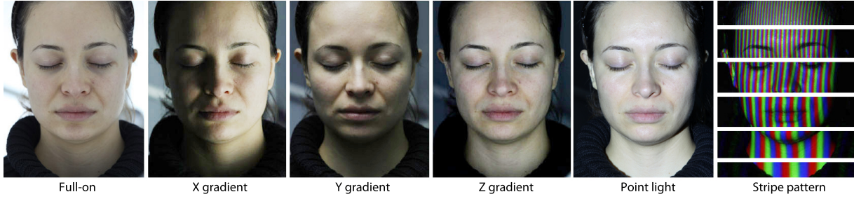
Figure 1: The controlled-light setup used for facial appearance capture.
