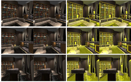
Fig. 8: This figure shows three example stereo frames from a rendered indoor sequence. The left images show the actual frames, whereas the right images the same images augmented with the wire-frame model of the scene placed using the estimated camera parameters. The results can also be found in the video accompanying this paper.
