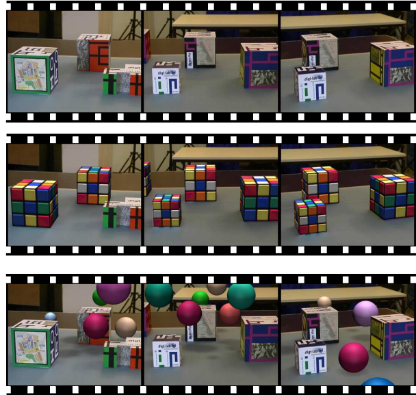
Figure 2. Reconstructed scene containing cubes on a tabletop. First row: original images of the scene. Second row: After modelling the scene, we can convert all cubes to Rubik's cubes. Third row: insertion of synthetic objects into the scene.
