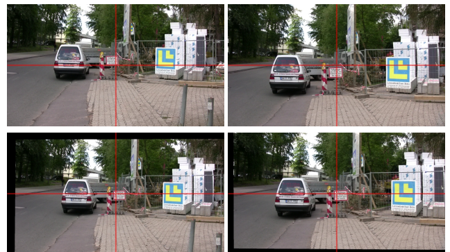
Figure 7: Example 3 - Original image sequence (top), result of stabilization by fixation (bottom).
